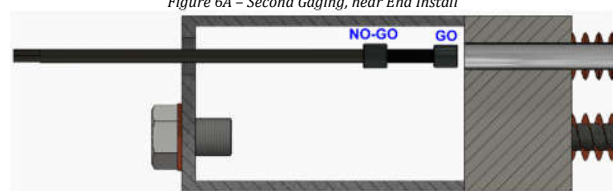
Figure 6B – Second Gaging, ACHE Install
