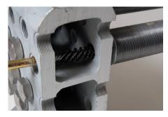
Plug Installation (Installing Pop-A-Plug® inside the tube sheet at depth)
