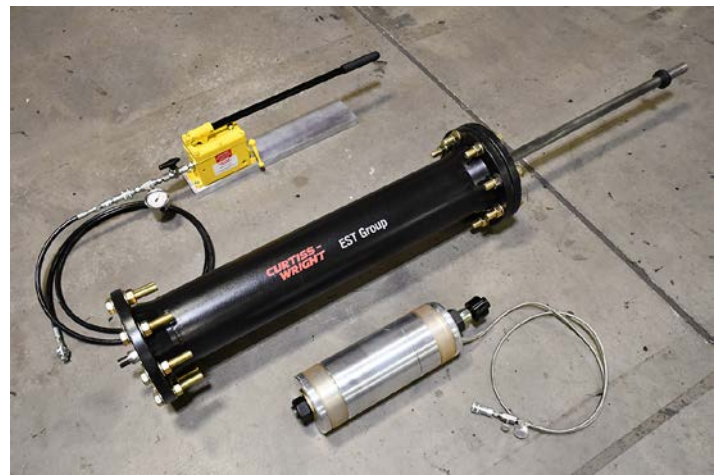
Figure 2 - The equipment required for the line isolation consisted of just three main components: a hydraulic hose line (top), the spool assembly (middle), and the hydraulically actuated DBB (bottom).
