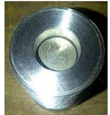
Figure 7. Test Coupon (10CrMo9.10) with P2-790-CR-SP-0611
