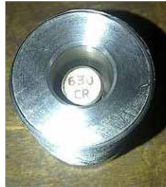
Figure 6. Test Coupon (10CrMo9.10) with P2-630-CR-SP-0611
